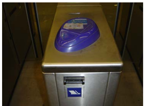
Magnetic paper and smart card ticket readers in one gate system (Lisbon, Portugal)
